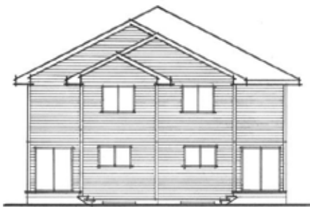
Inappropriate High Visibility Rear Treatment 'Craftsman'
