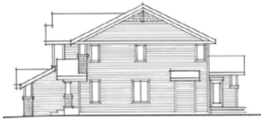
Inappropriate Corner Treatment 'Craftsman'
